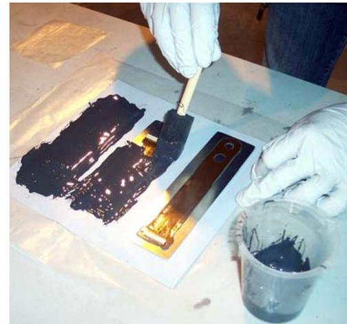
Sealant removal for data acquisition
