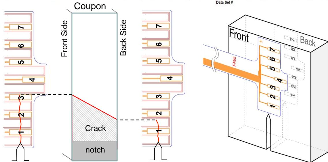
***This test proved that either in continuous on-board monitoring mode or when using portable data logger on the ground, surface-breaking cracks provided a large, reliable response compared to drift and other error sources***
