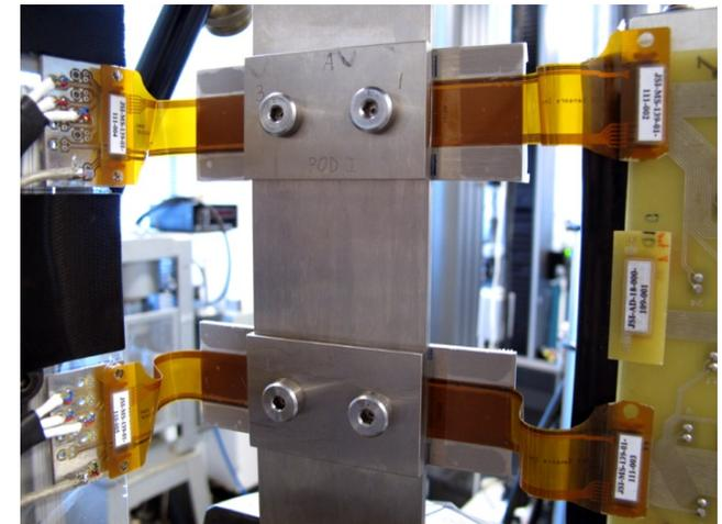
Note that on the same coupon with holes machined in the same manner, under the same load, there is still a very large scatter in the time to crack initiation.
