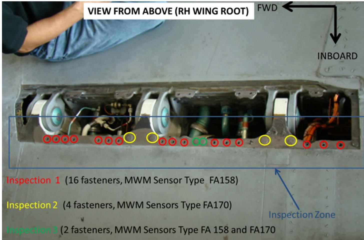
**Inspection 1** (16 fasteners, MWM Sensor Type FA158)
